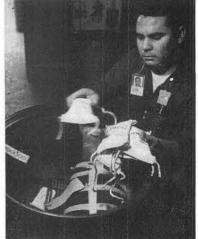
SACKS of desiccant are packed around electronic gear destined for long-range shipment by Gabriel Chavez (4624-2). They'll absorb stray moisture in metal packing container, reduce chance of possible humidity contamination.
